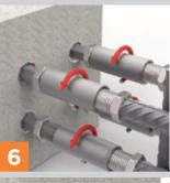
Rotate the couplers towards the assembly rebars until they start engaging.
