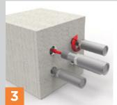
Insert and rotate the studs. Check that the studs are screwed up to the threaded end of the 1st phase fixed rebars without being blocked.
