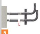
Check the distance "L" between the studs and 2nd phase rebars. The maximum distance allowed is indicated in table 6 below.
